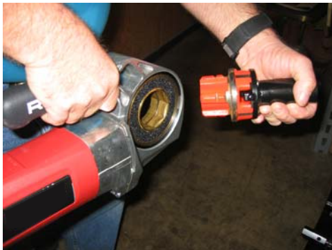
Adaptor fits onto power winder
