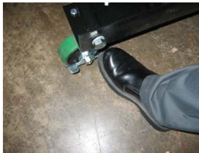
Unlock brake and roll into position
