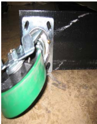
WRONG plate direction
