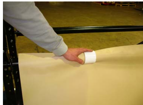
Place one clip retainer approx. 1/4 toward center from each end.
