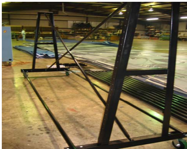
Both Spacer tubes and cross braces attached to A-Frame ends.
